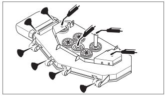
Figure 19. Deck Lubrication
